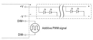
"DO NOT connect "DIM- to -V"
