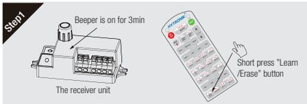
Short press "Learn/Erase" button on RC to the receiver to activate pairing mode, and the receiver unit will beep once every second for 3min.
