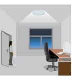
With insufficient natural light, the sensor switches on the light automatically when presence is detected.
